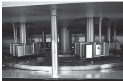
Rotating substrate table at the chamber top for 10 substrates (in situ combinable with five masks) + 4 high-temperature thermal radiation heaters on the rear
