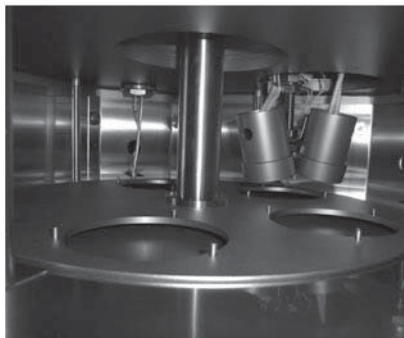
Coaxial hollow shaft drive for eccentric rotation and positioning of several substrates, with separate shutter table
