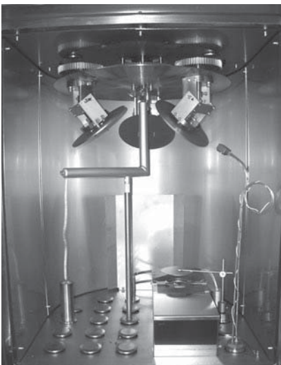
Chamber bottom: electron beam evaporator with sixfold rotating crucible Chamber top: planetary drive for substrate rotation
