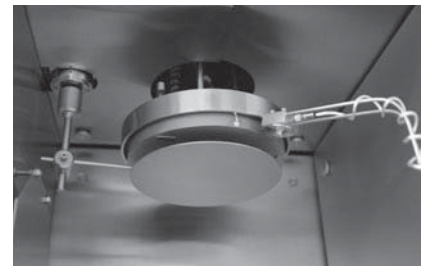
Rotating, resistively heated substrate table with shutters and thin film gauge head
