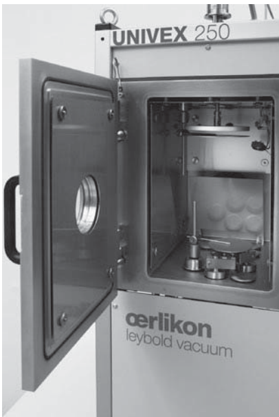
Chamber bottom: double thermal evaporator with source shutter Chamber top: rotating substrate table with substrate shutter
