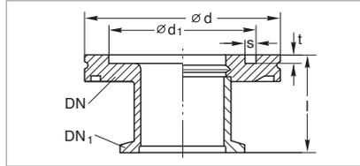
Dimensional drawing for the adaptors-reducer ISO-K – ISO-KF;
