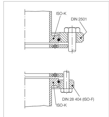
Comparison: Clamp flange with collar flange to DIN EN 1092-1 and clamp flange with collar flange to DIN 28 404; ISO-F
