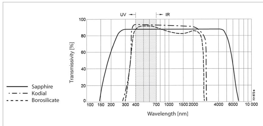
Optical transmissivity for the CF observation windows
