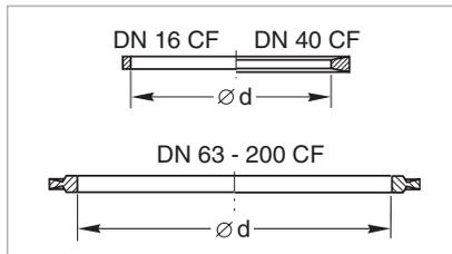
Dimensional drawing for the profiled gaskets without support ring
