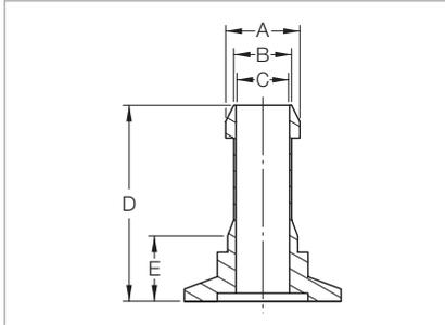
Dimensional drawing for the ISO-KF nipples
