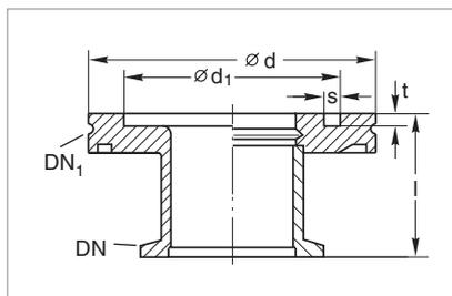
Dimensional drawing for the adaptor reducers ISO-KF – ISO-K;
