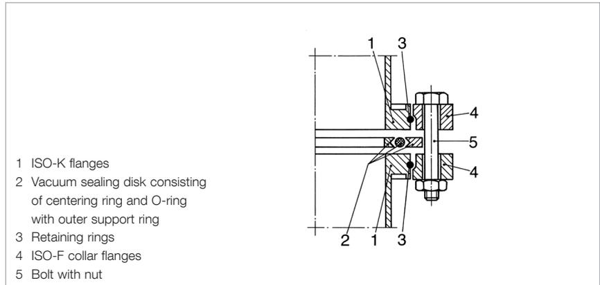
Clamped flange connection with collar flanges
